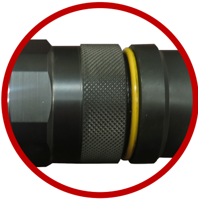
Incorrect Coupling—O-Ring Exposed
