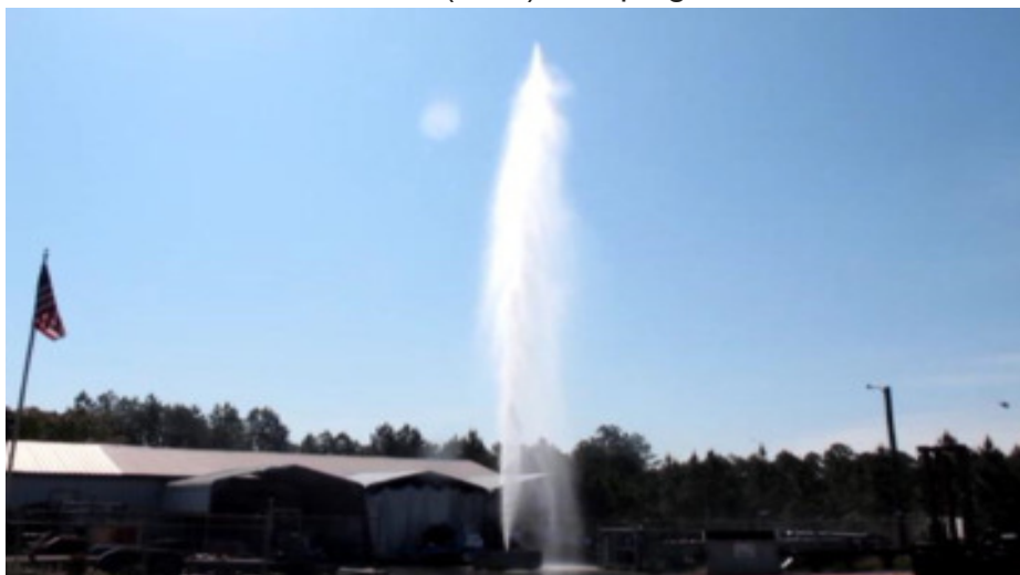
75' Fountain of water from a 3" Tank Cleaning Pump and a 1" discharge coupling
