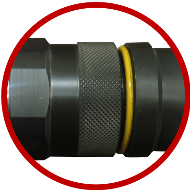
Incorrect Coupling—O-Ring Exposed
