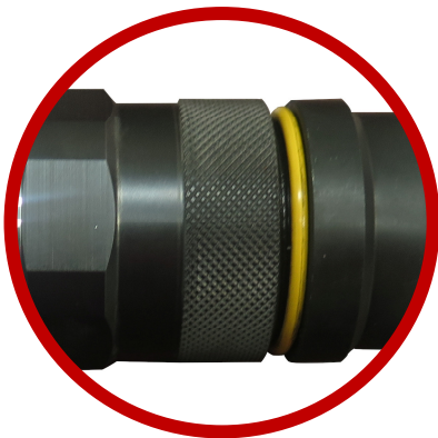
Incorrect Coupling—O-Ring Exposed
