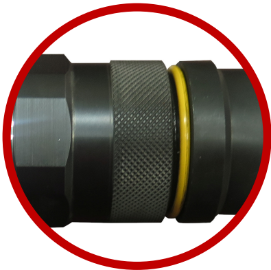
Incorrect Coupling—O-Ring Exposed
