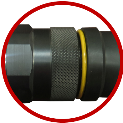
Incorrect Coupling—O-Ring Exposed
