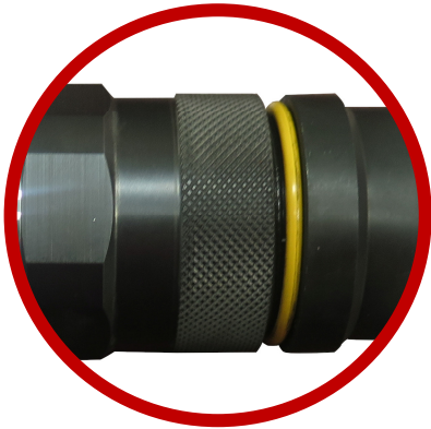
Incorrect Coupling—O-Ring Exposed
