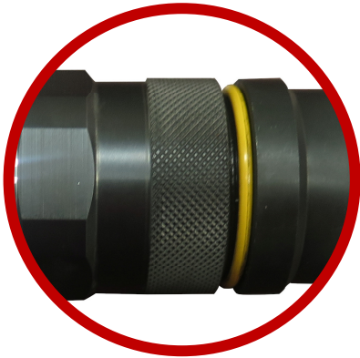
Incorrect Coupling—O-Ring Exposed
